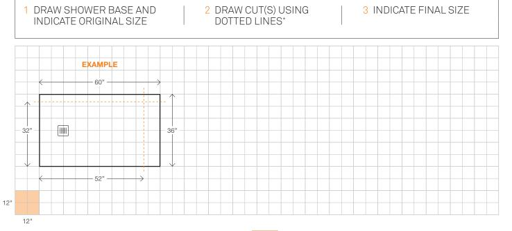
\*End-drain and off-set models: cuts are not possible on the side closest to the drain.
